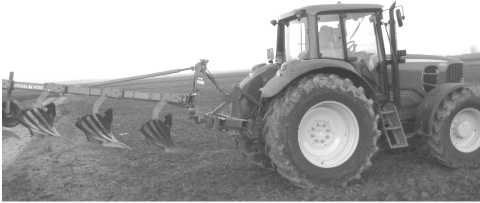
Figure 4. Draft measuring system (tractor+three-point-hitch device) and tested plow (slatted moldboard plow)
