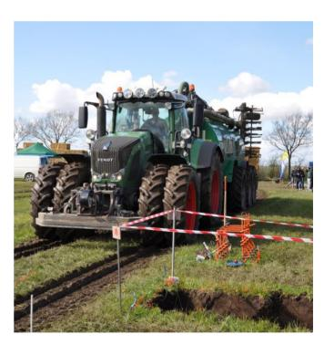
Tractor plus slurry tanker (>50 Mg in total) approaching the area where soil stress is being measured (photo by Martin Thorsøe).
